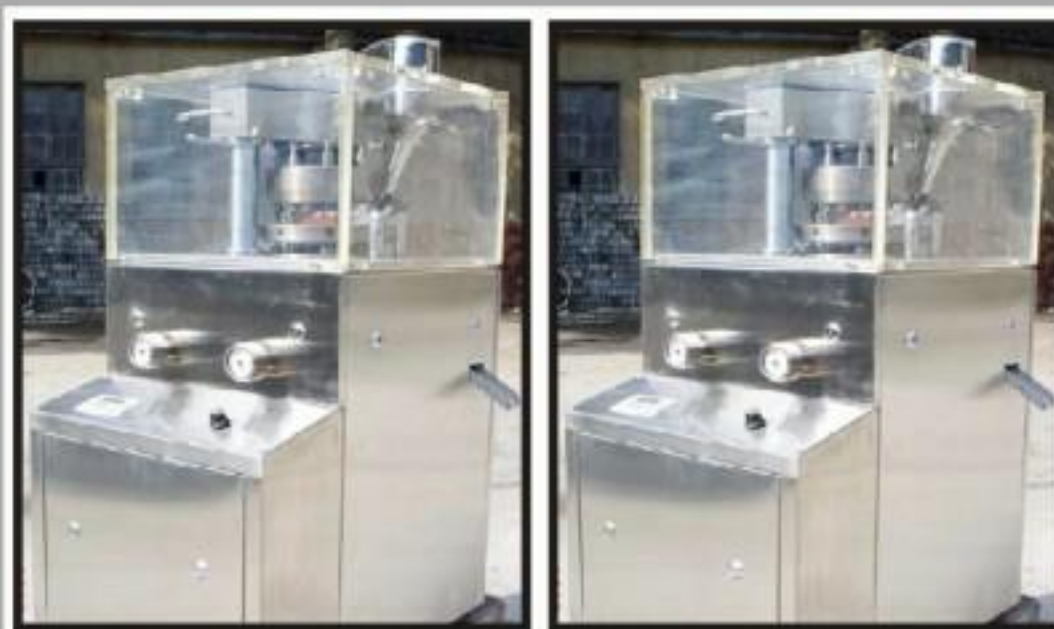
ZP-33 Tablets Compressing Units are in Operation
